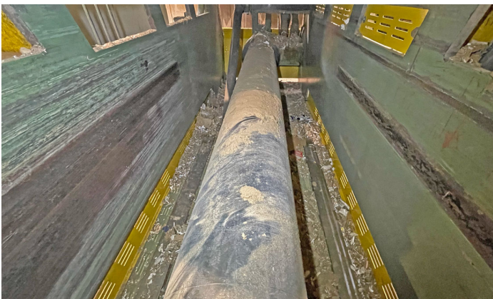
The main hydraulic cylinder is in good condition and tight
