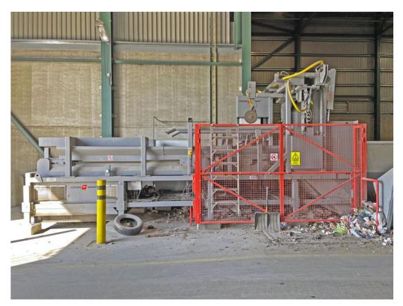
It is a complete line for opening pressed bales made of RDF/MSW, paper, cardboard.
