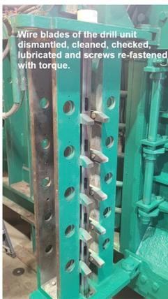
Wire blades of the drill unit dismantled, cleaned, checked, lubricated and screws re-fastened with torque.
