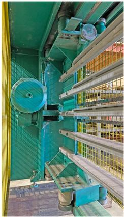
All needle bars, incl. needle heads with wire rollers and bearings completely renewed
