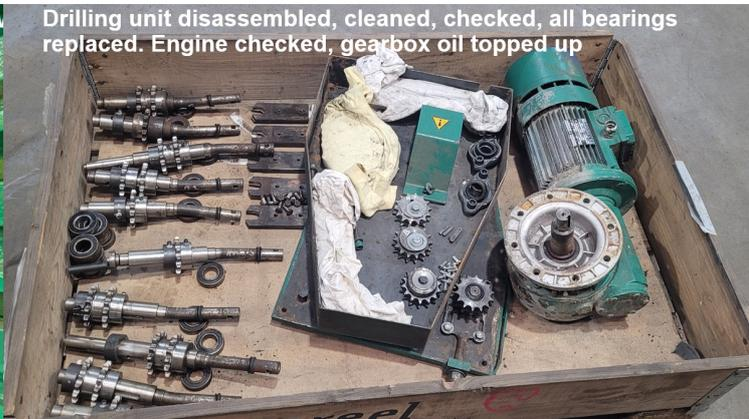
Drilling unit disassembled, cleaned, checked, all bearings replaced. Engine checked, gearbox oil topped up
