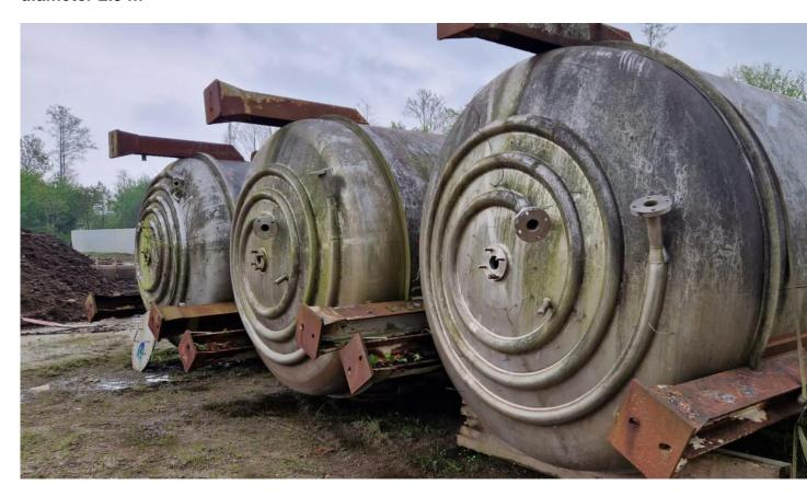
We offer you 3 pieces of V2A steel tanks, tank height without stands 9.6 m, tank height with stands 10 m, diameter 2.5 m. Unfortunately, type plates are not available, further details are also missing. Water was last stored in the tanks before they were dismantled. More information is not known. You can inspect the tanks at our premises in Scheemda, the Netherlands.
