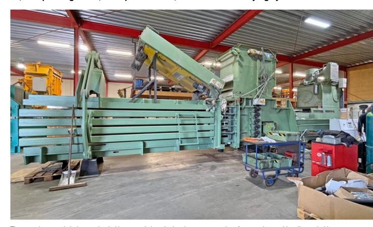
The press is currently being overhauled in our workshop. In the photos you can therefore see the machine dismantled in parts, where individual assemblies and cylinders are missing. These will be reassembled after the overhaul work and the press will be tested in manual and automatic mode. We expect the machine to be ready for operation in November.
