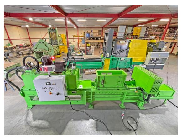
According to the manufacturer, this machine is suitable for pressing tin cans, metal sheet offcuts, sheet steel as well as aliminium, brass and copper waste and was completely overhauled in our workshop.
