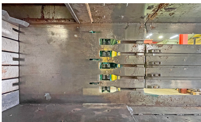
All needle bars, incl. needle heads with wire rollers and bearings completely renewed
